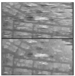
Figure 5. Applying dynamic programming algorithm to stereo pair of fig. 4 results in the DEM shown left. Applying a median filter reduces blunders significantly (right).
