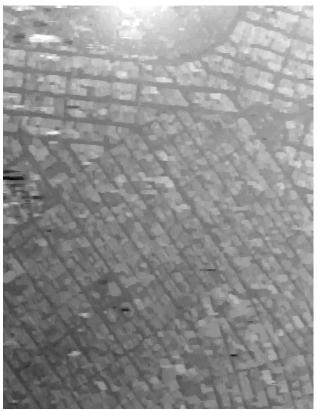
Figure 19. DEM of a larger area out of the Ikonos image Athens. fig. 4 can be found in the upper left corner. Urban structure is fairly good observable to distinguish between streets and build up objects (or high vegetation like trees)
